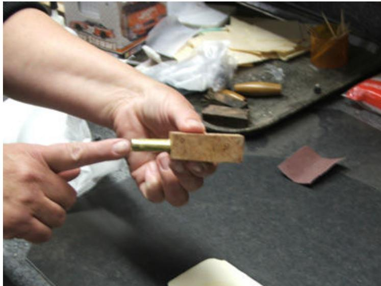
.After pre-fitting the brass tube (to make sure it fits), apply a generous portion of 5-minute epoxy to your tube. Insert the tube into your wood pen blank twisting as you go in to help spread the glue evenly. Try to make sure no excess glue gets inside the brass tube.
