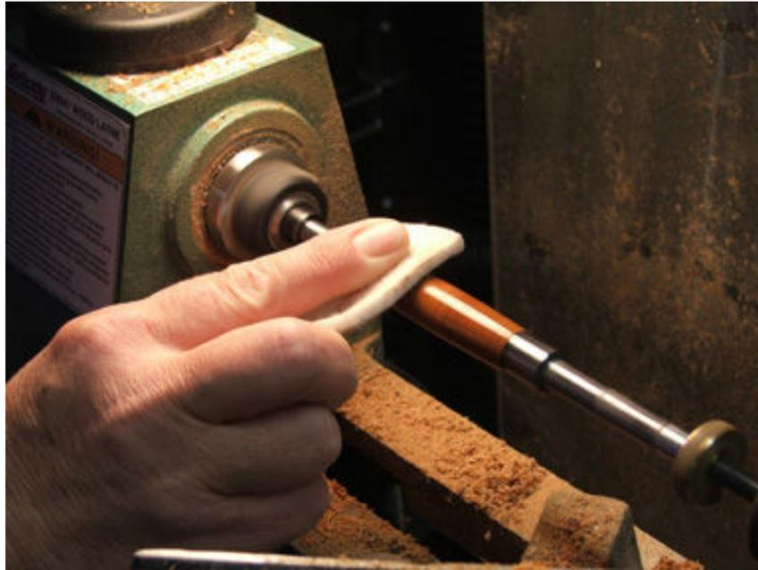
Use a buffing pad between coats. If wax ridges appear, try buffing pad to remove. If not successful, you may have to use the white 3-m pad which will require you to reapply the polish and wax again..
