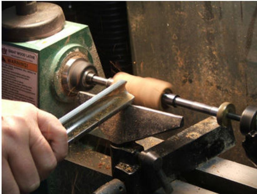
.Rough your pen blank to a cylinder using a tool you feel comfortable with. Gouges work best for this purpose.
