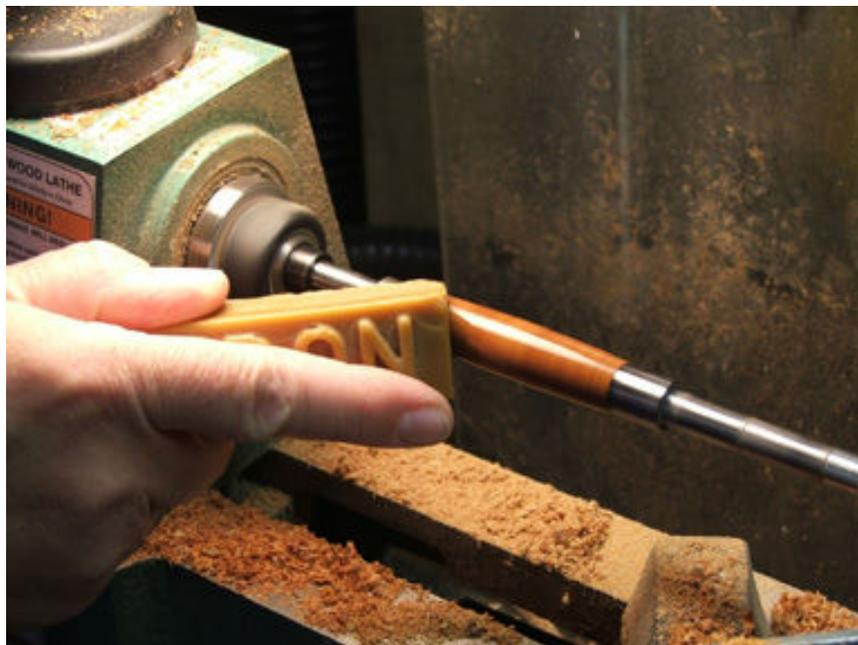
.Apply 3-4 coats of carnuba wax. Constant horizontal movement of bar will help prevent wax ridge buildup.
