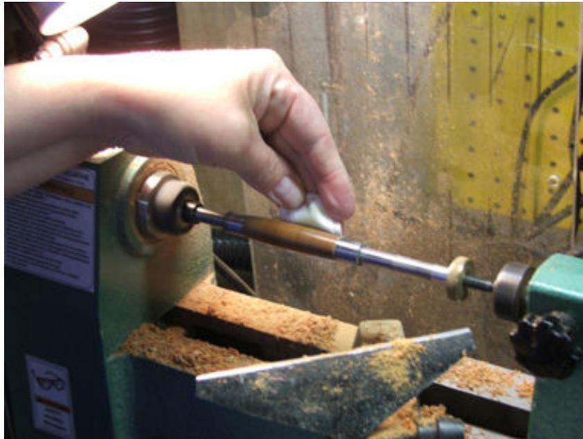
If you are happy with your sanding, apply 2 coats of friction sanding sealer with a small lint free rag. This will raise the grain and remove any fine saw-dust in the pores of the wood.
