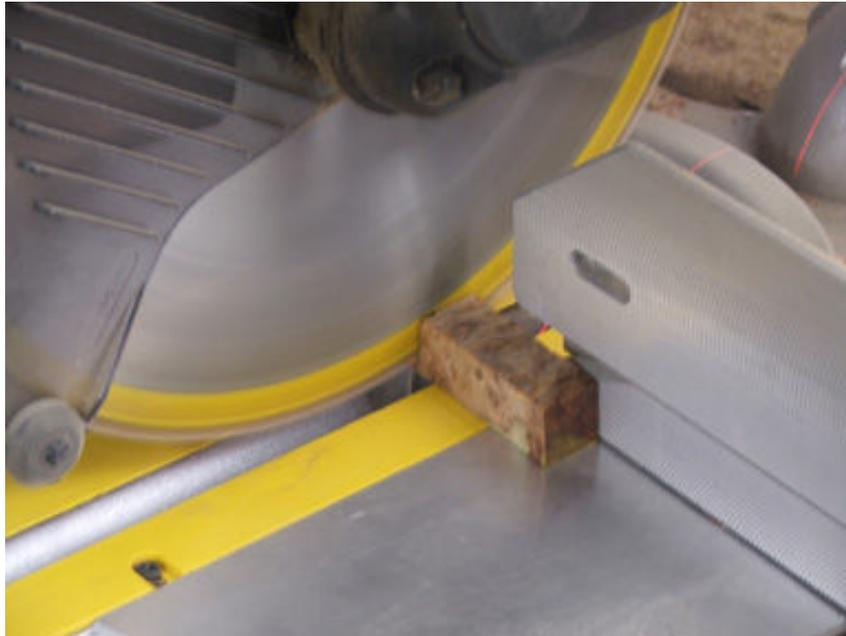
Cut the pen blank to size with a band saw, scroll saw, chop saw, table saw, or a hand saw for that matter....use what you are comfortable with.
