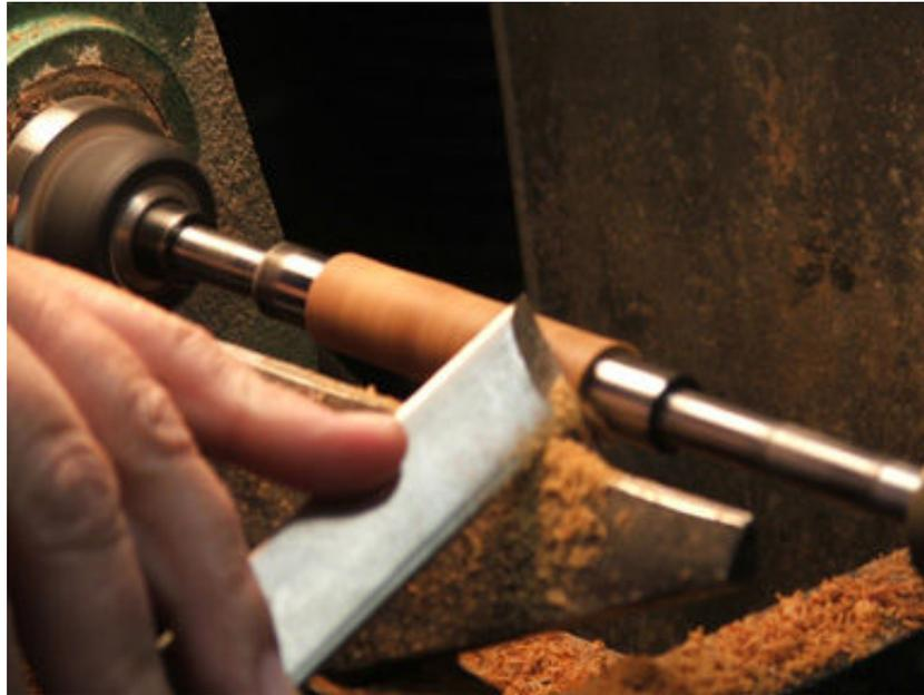
Turn the blank down to the bushing. **REMEMBER**, you can always sand a little more off, but you can't put it back on! Shape the pen barrel to your liking.
