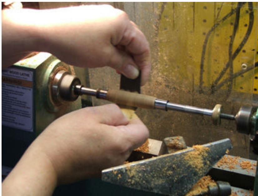
.Sand the pen barrel going through the grits. In between grits wipe away any excess sawdust and check for sand paper "rings". If they appear, sand horizontally (with the lathe off) before proceeding onto the next grit.
