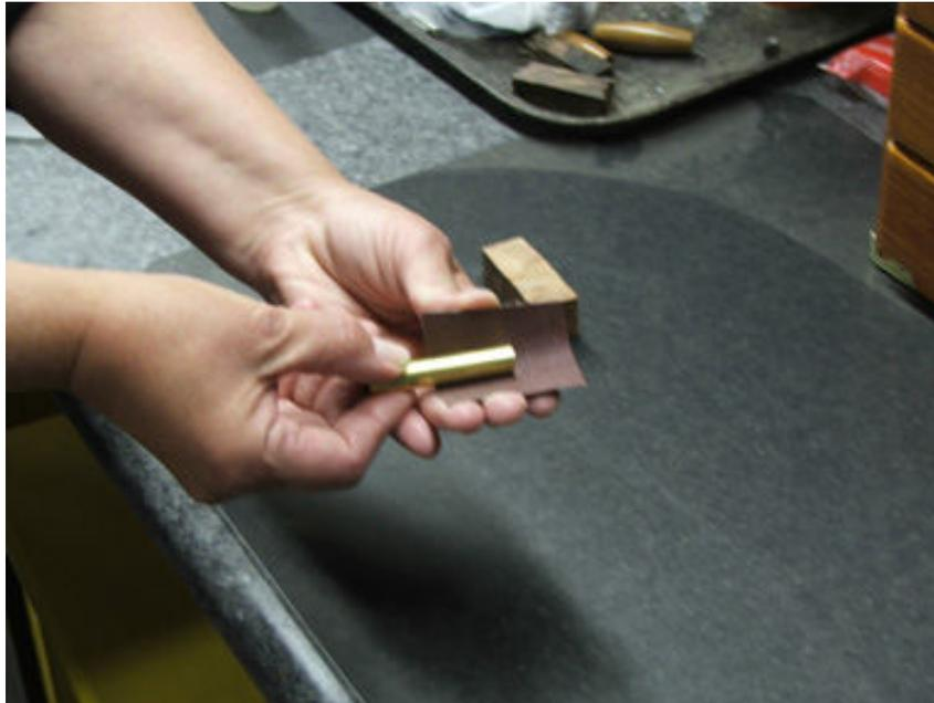
Using a coarse grit sand paper (80 will do) to sand the brass tube. The Small grooves the sanding leaves will give the glue something to bond to.
